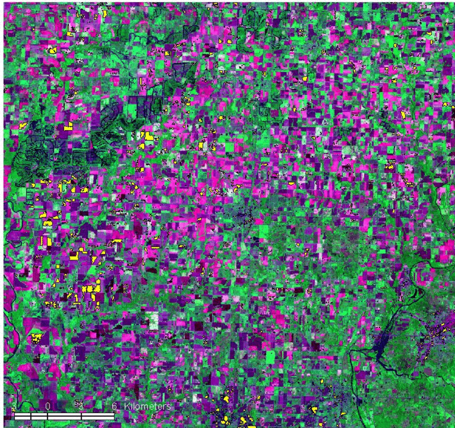
Figure 4. Supervised classification showing mine waste/tailings land cover in yellow. Landsat TM image of Cherokee County, Kansas (June 27, 1992). Bands 7-4-2 coded red, green, and blue.
